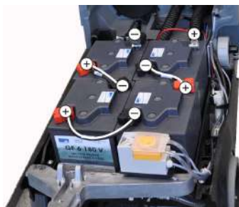
Monteringskisse for 4 batterier
