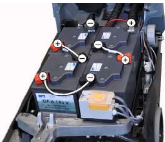
Installation sketch for 4 batteries
