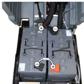
Installation sketch for 2 batteries
